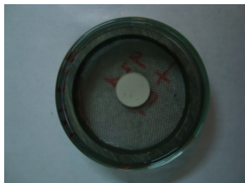
Figure 1: Device used to measure water uptake and swelling of Carbopol polymers
