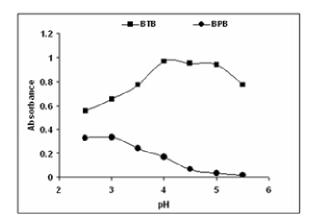
Figure 2. Effect of pH on ion pair complexes of domperidone.
