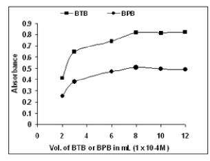
Figure 4. Mole ratio study of drug-dye system (Domperidone-BTB and domperidone-BPB ion pair complexes).
